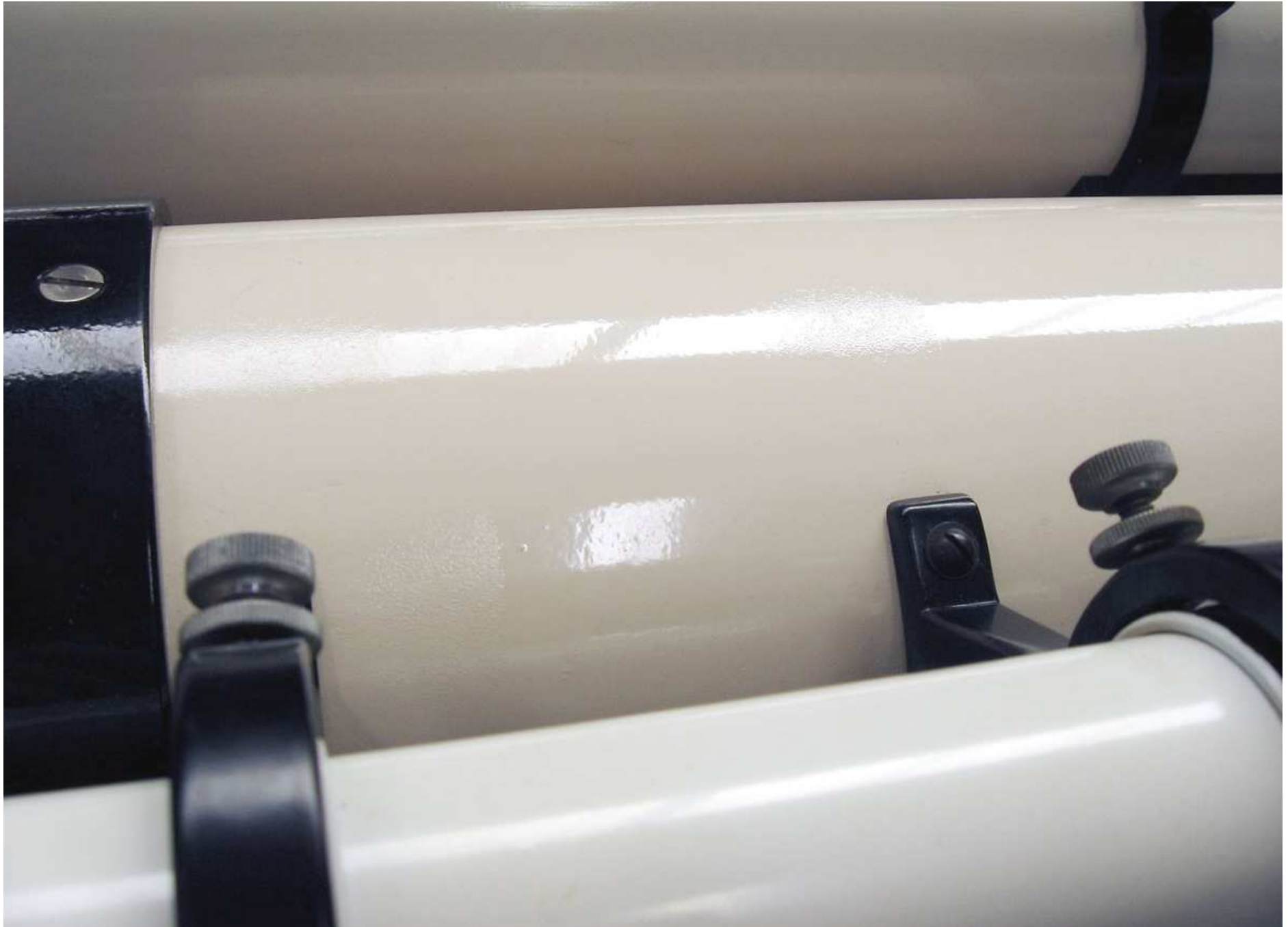
IMG_1659: 6" OTA trying to show some paint imperfections and marks; guide scope on bottom of picture
