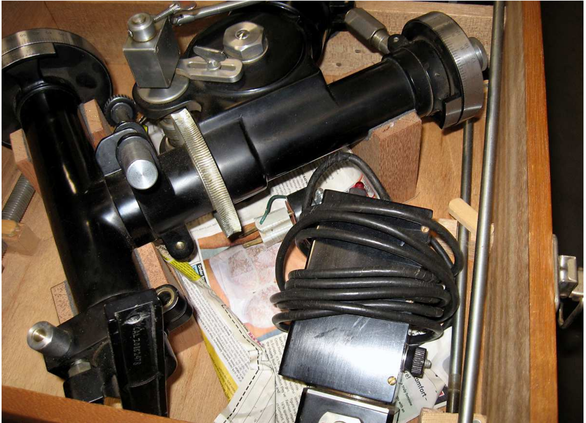
IMG_1633: closer view of equatorial head and Unitron clock-drive unit
