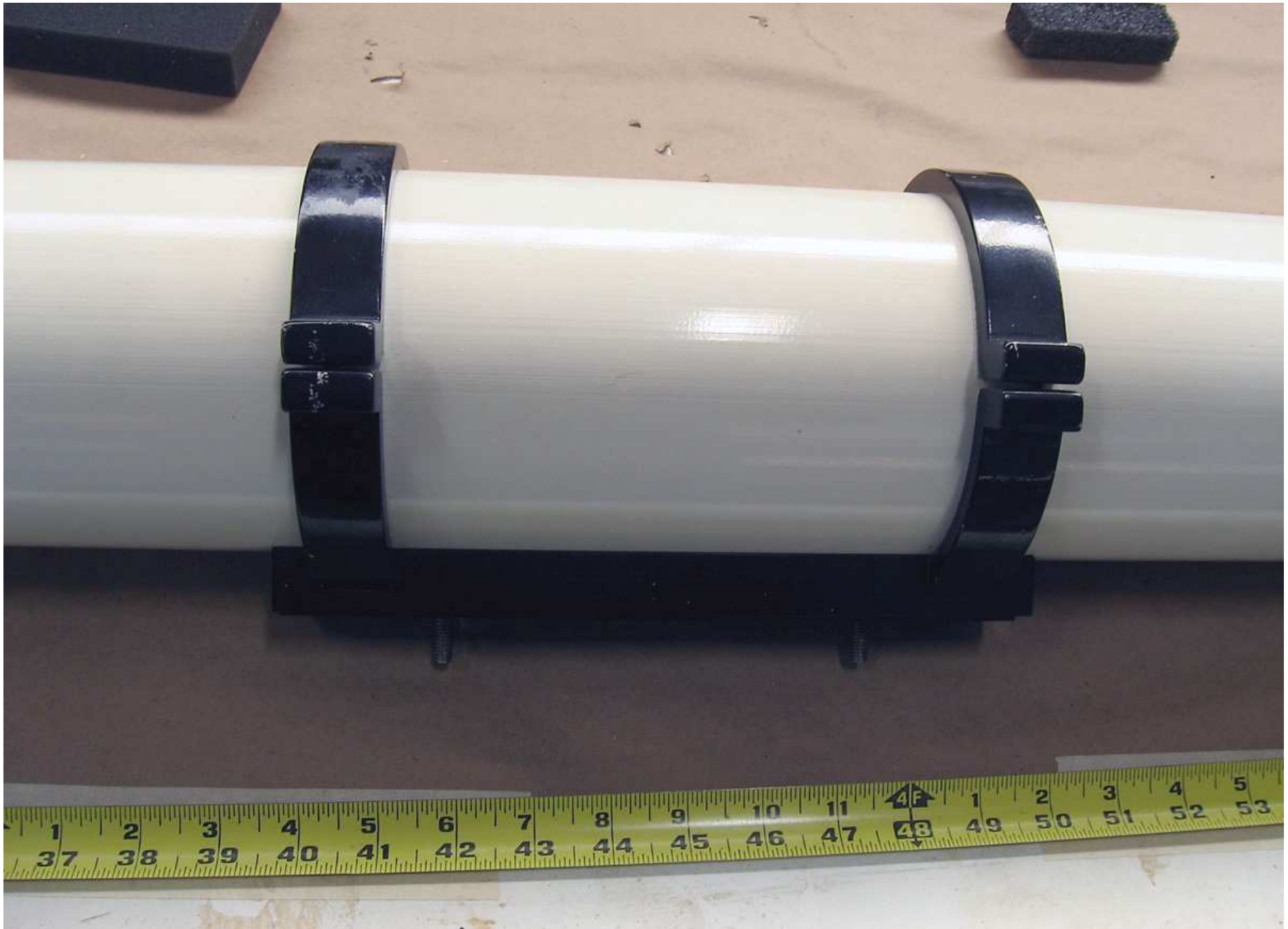
IMG_1674: Tube rings and mounting block on 5" OTA. Note lengthwise striations on OTA, some scuffing on rings.
