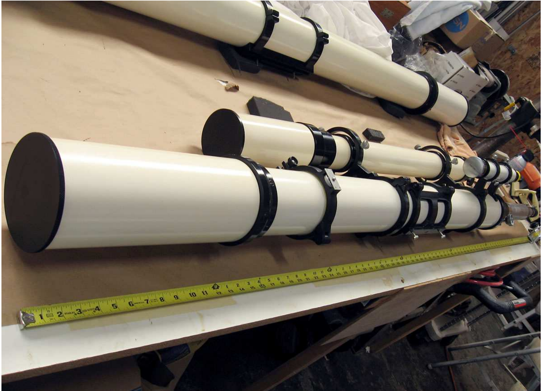
IMG_1683: 4" OTA, 3" Guide Scope, Unitron 40mm finder and ring for camera attachment. 5" OTA in background.
