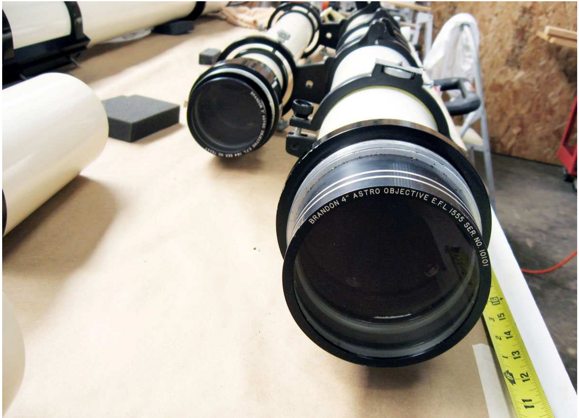
IMG_1694: 4" OTA and 3" Brandon Objective guide scope. I do not know if Unitron used Brandon objectives in some of their scopes.
