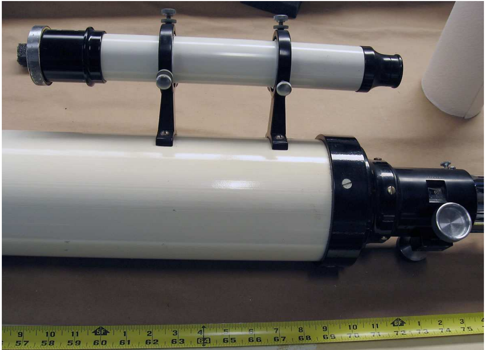
IMG_1673: 5" OTA, 10x-40mm Unitron finder. Note paint flakes on OTA and striations that run length of the tube, pitting on finder cap.
