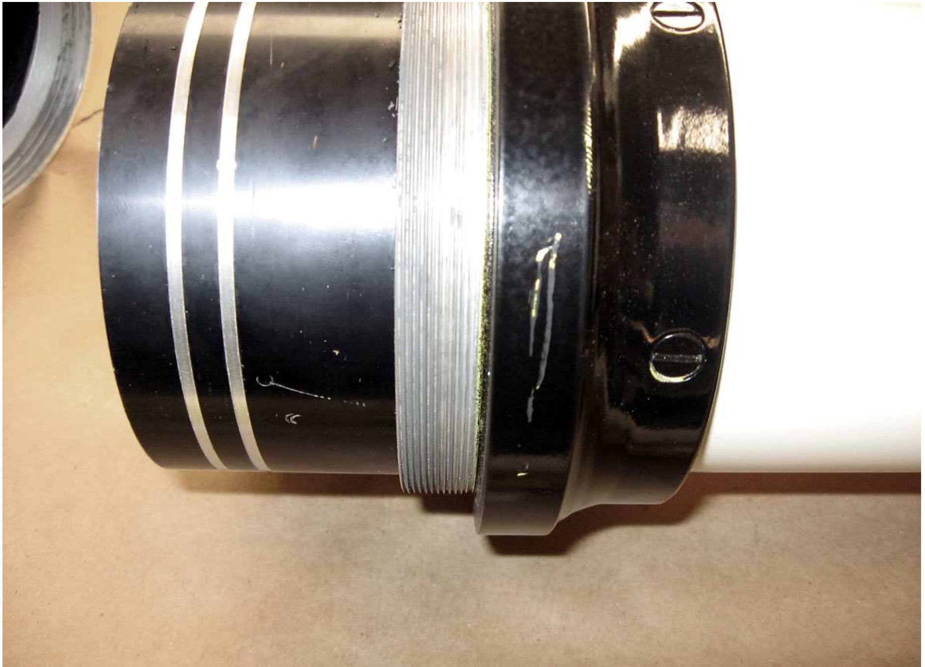
IMG_1692: 4" OTA, side view, scratch in lens cell shows brass. This may answer why this OTA is so heavy.
