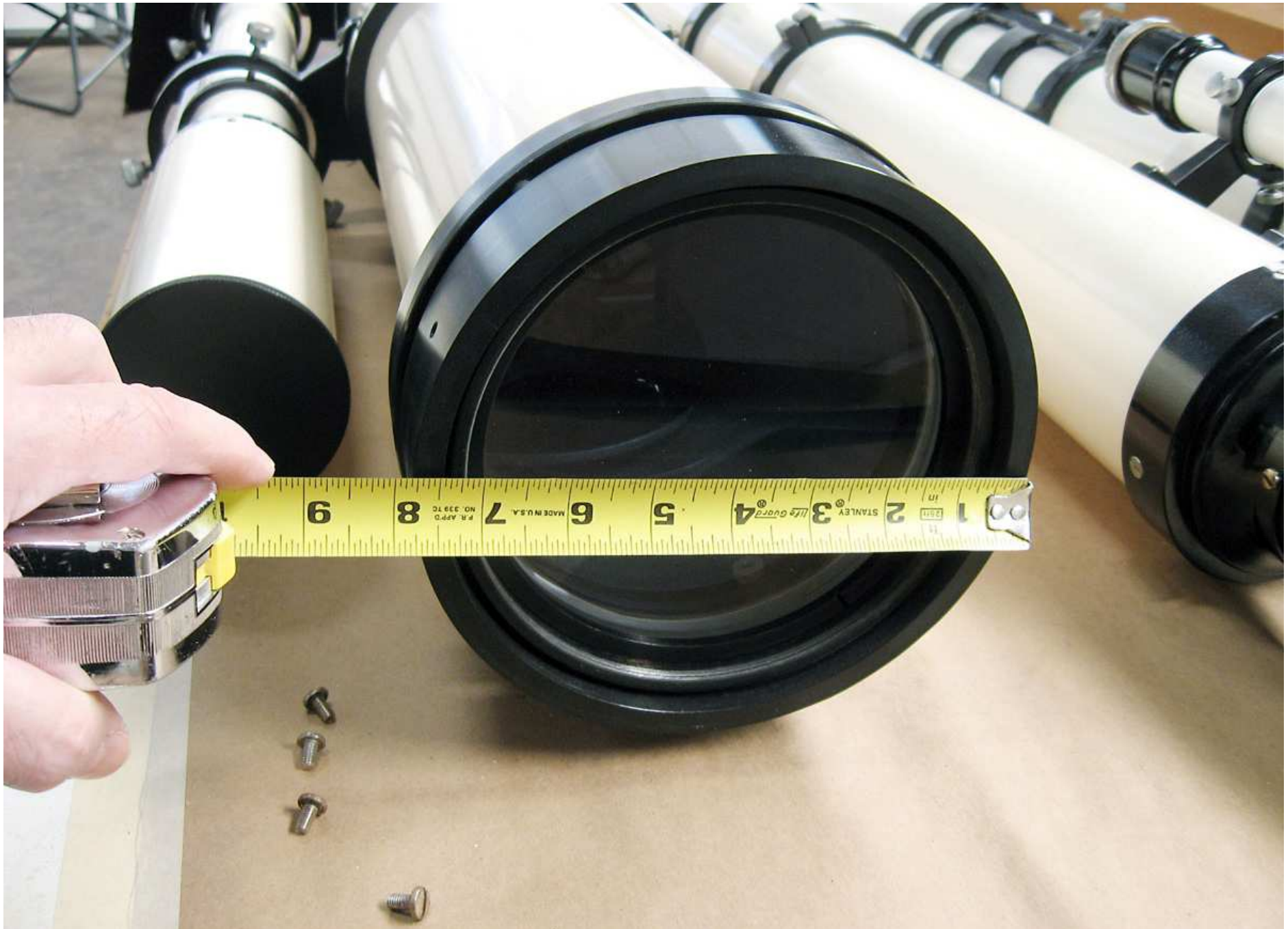
IMG_1661: 6" Objective, couple of dust particles inside, coatings are present, no scratches or marks observed
