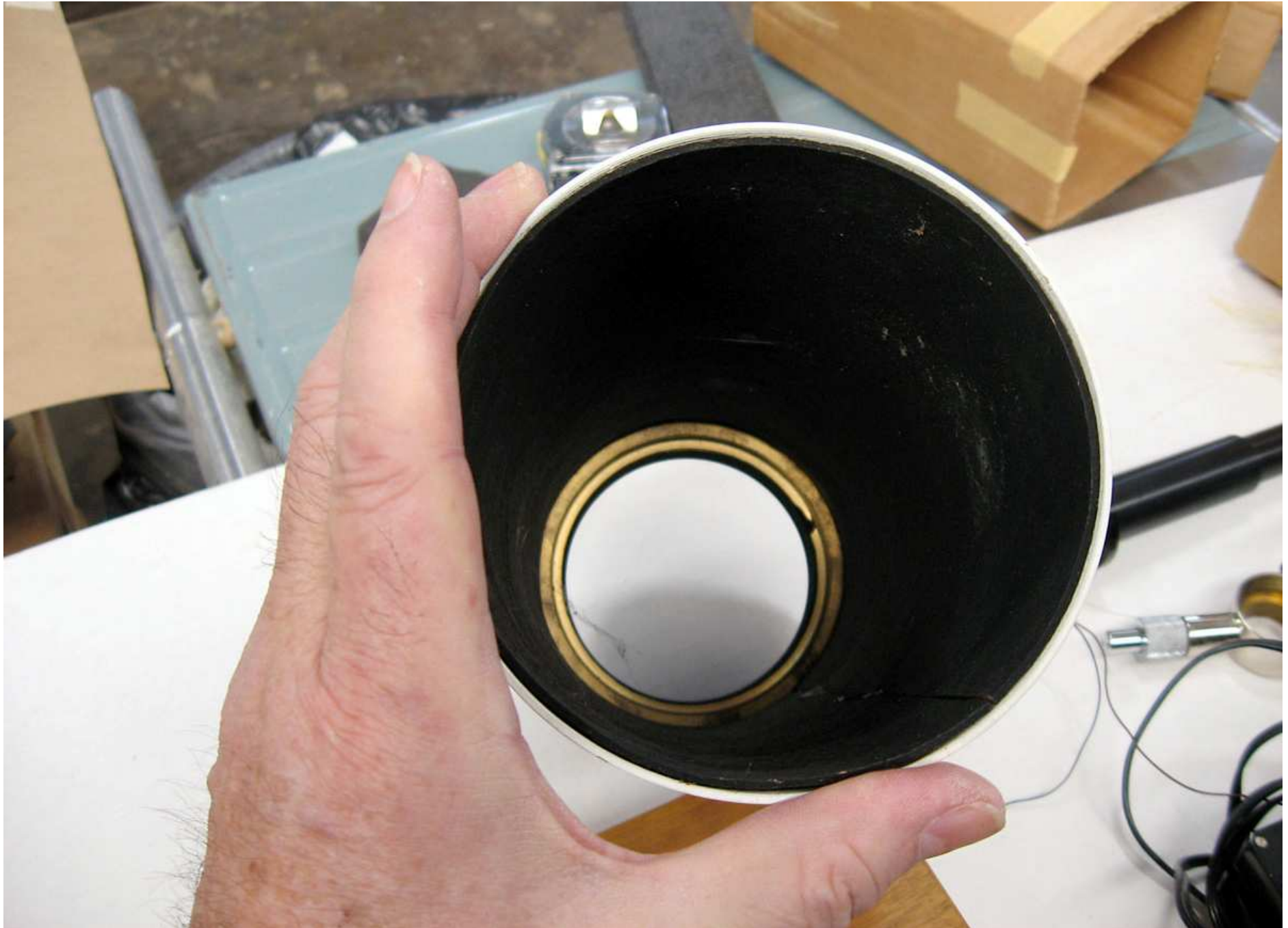
IMG_1704: Dew shield for 4" scope with brass fitting for objective
