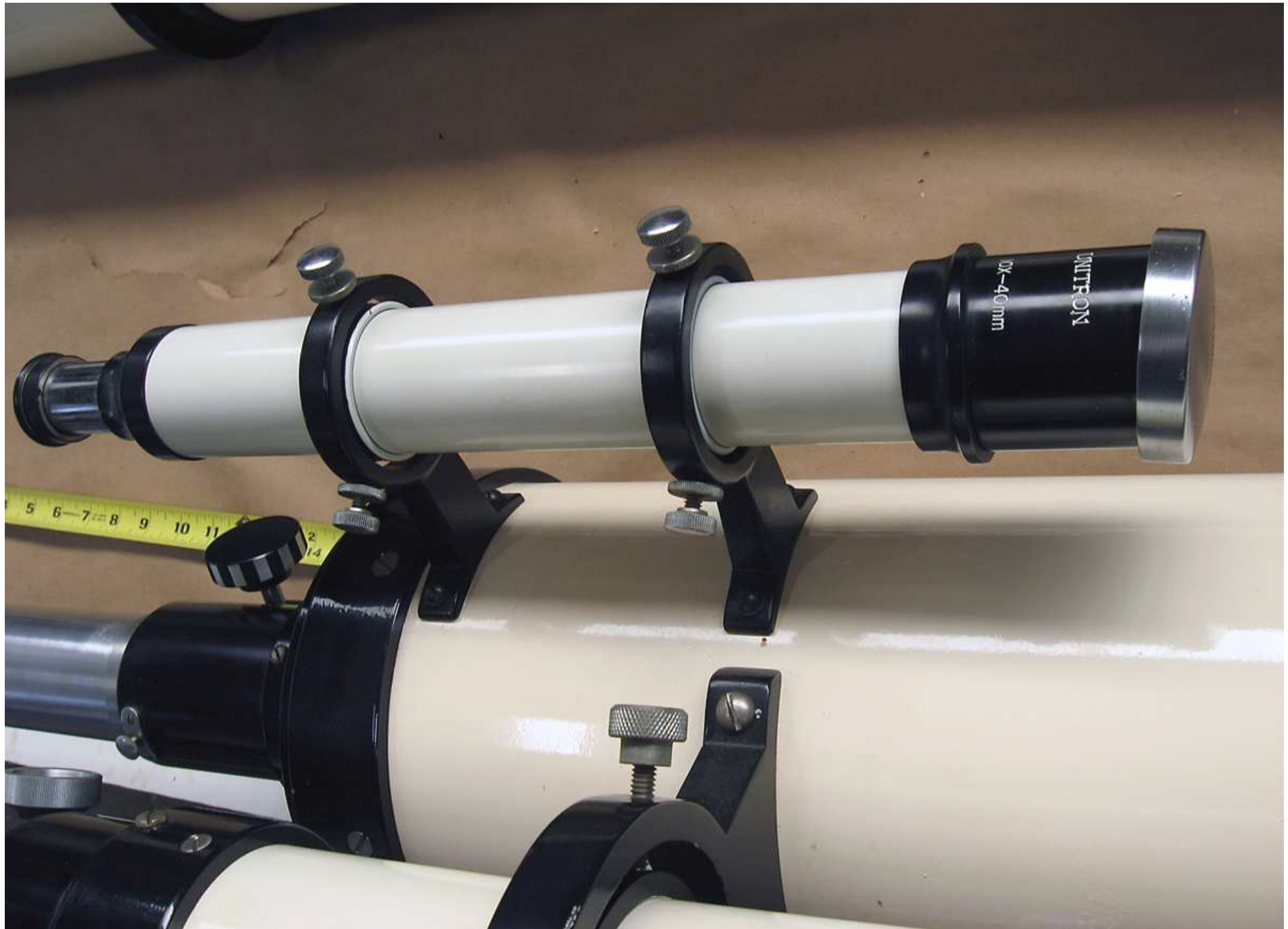
IMG_1653: Unitron 10x-40mm Finder Scope attached to 6" OTA. The metal dew cap has some pitting to chrome plate.
