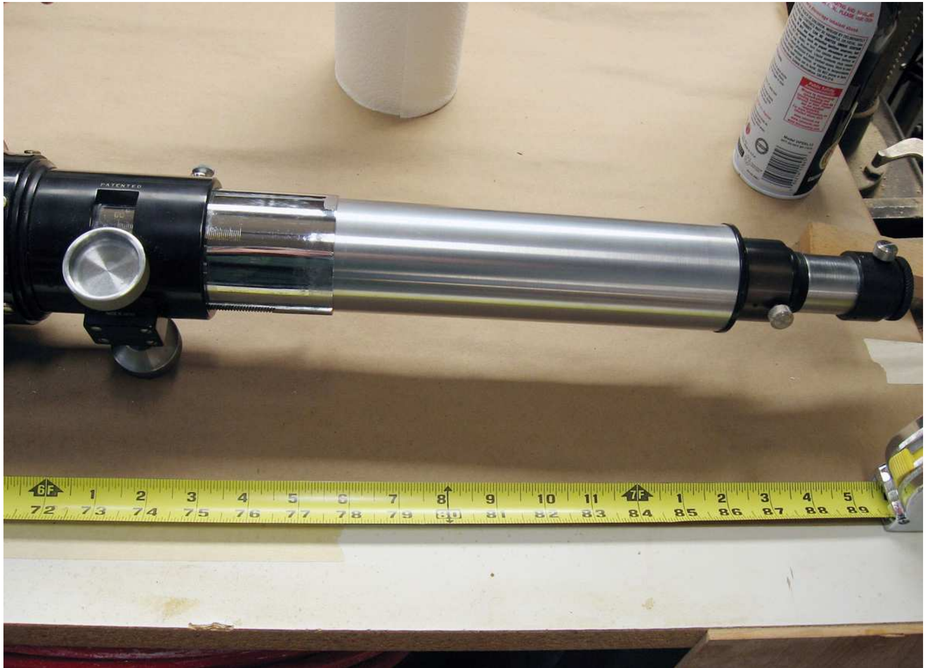
IMG_1672: Unitron Focuser on 5" OTA, extended. Note window for precise focus measurements.
