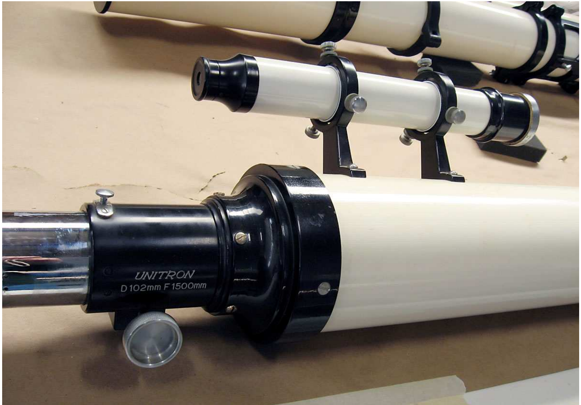
IMG_1680: 5" OTA Focuser opposite side as photo # 1672. The entire OTA is in very nice condition with 10x 40mm Unitron finder. The focuser is a D102 F 1500, but the OTA and lens is 5"; have no idea who made the objective or if this is a complete Unitron scope.
