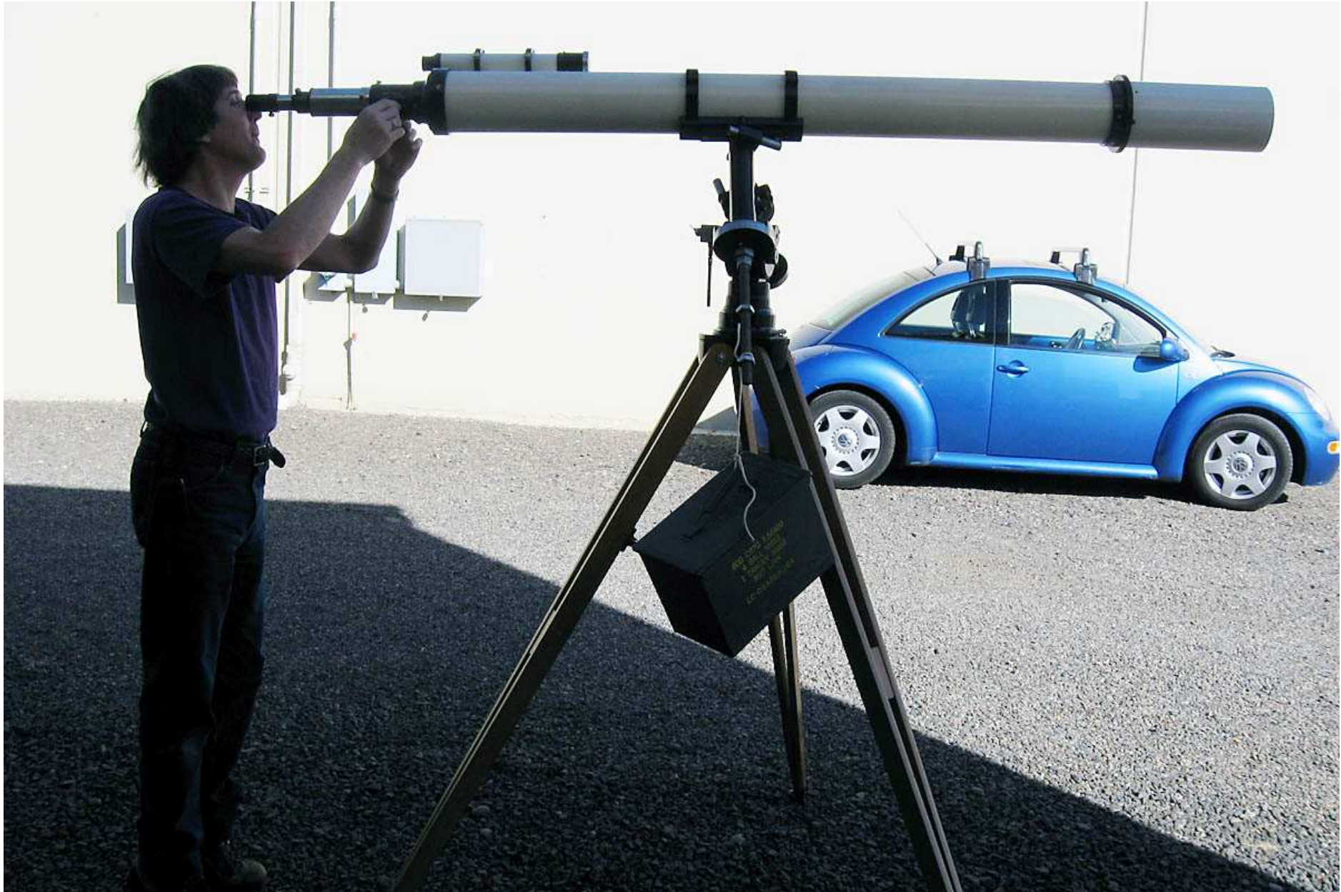
IMG_1592: We put all three OTA's, 4", 5" and 6" on the mount and they reached focus and the image seemed clear and good. The 5" OTA is pictured above on the mount and tripod in the pictures. We had to improvise a counter weight.
