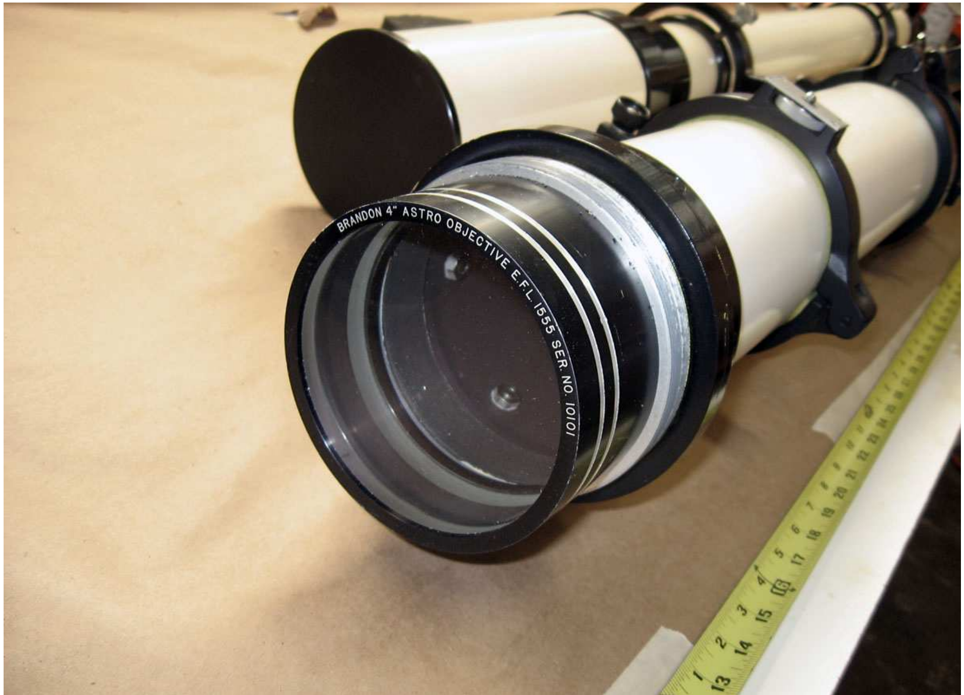
IMG_1690: 4" OTA with dew shield off, Brandon 4" cell. Objective is free of any visible marks or scratches, very little dust.
