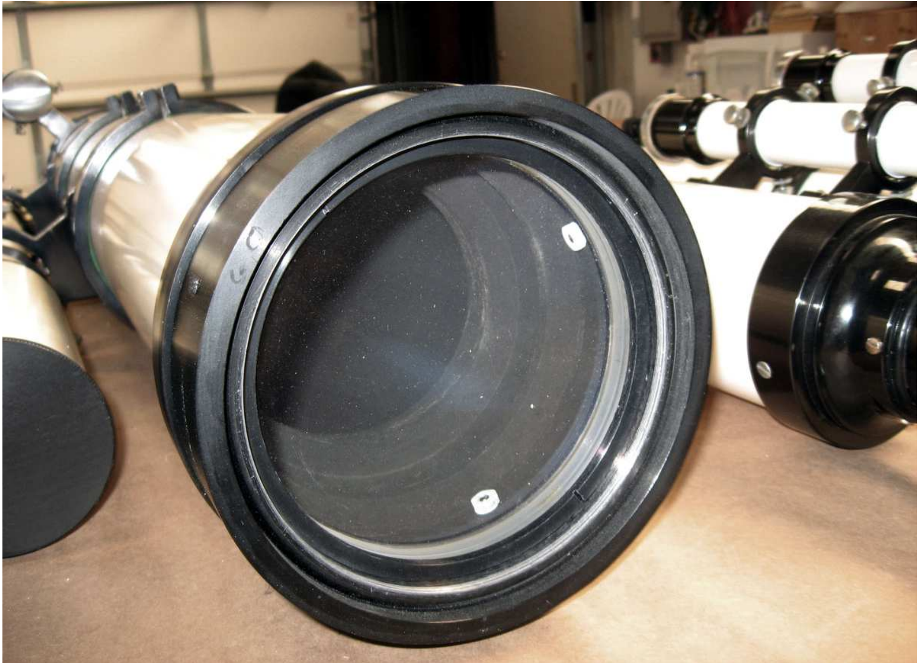
IMG_1662: Bright light to show no marks on 6" objective but some dust inside. Almost none on outside; we did not clean any optics.
