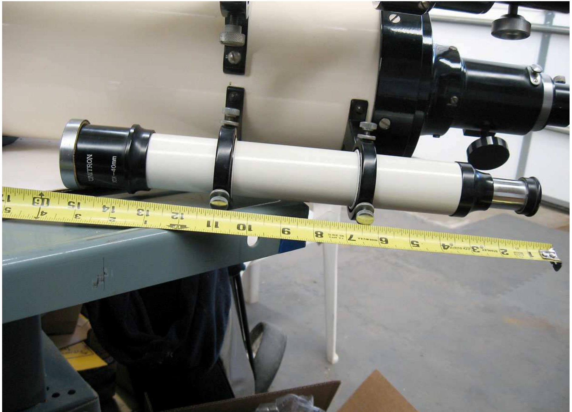
IMG_1669: Unitron finder scope attached to 6" OTA
