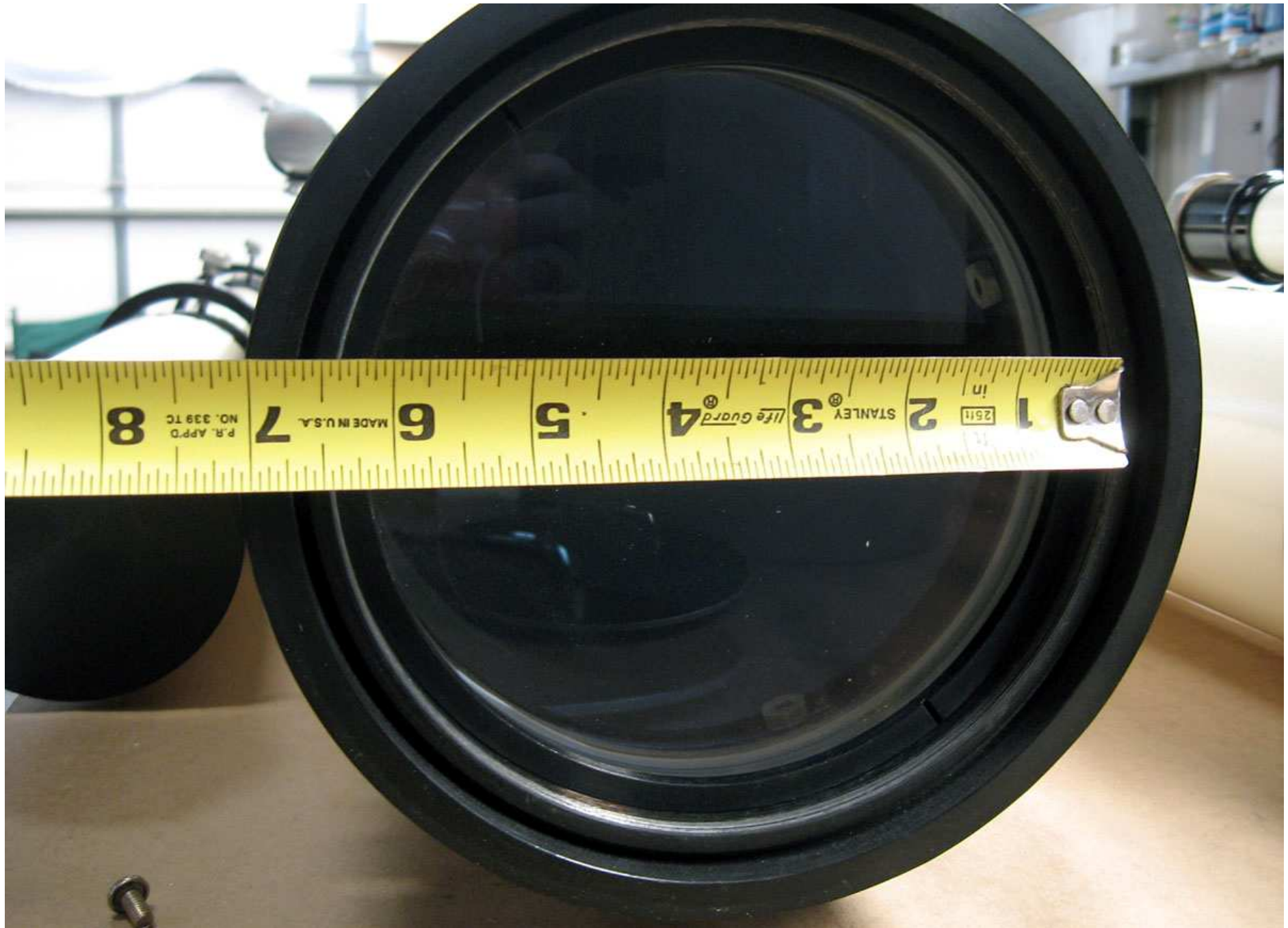
IMG_1663: Normal light image of 6" objective to show coatings and some internal dust. Did not take objective cell out; nor cleaning.
