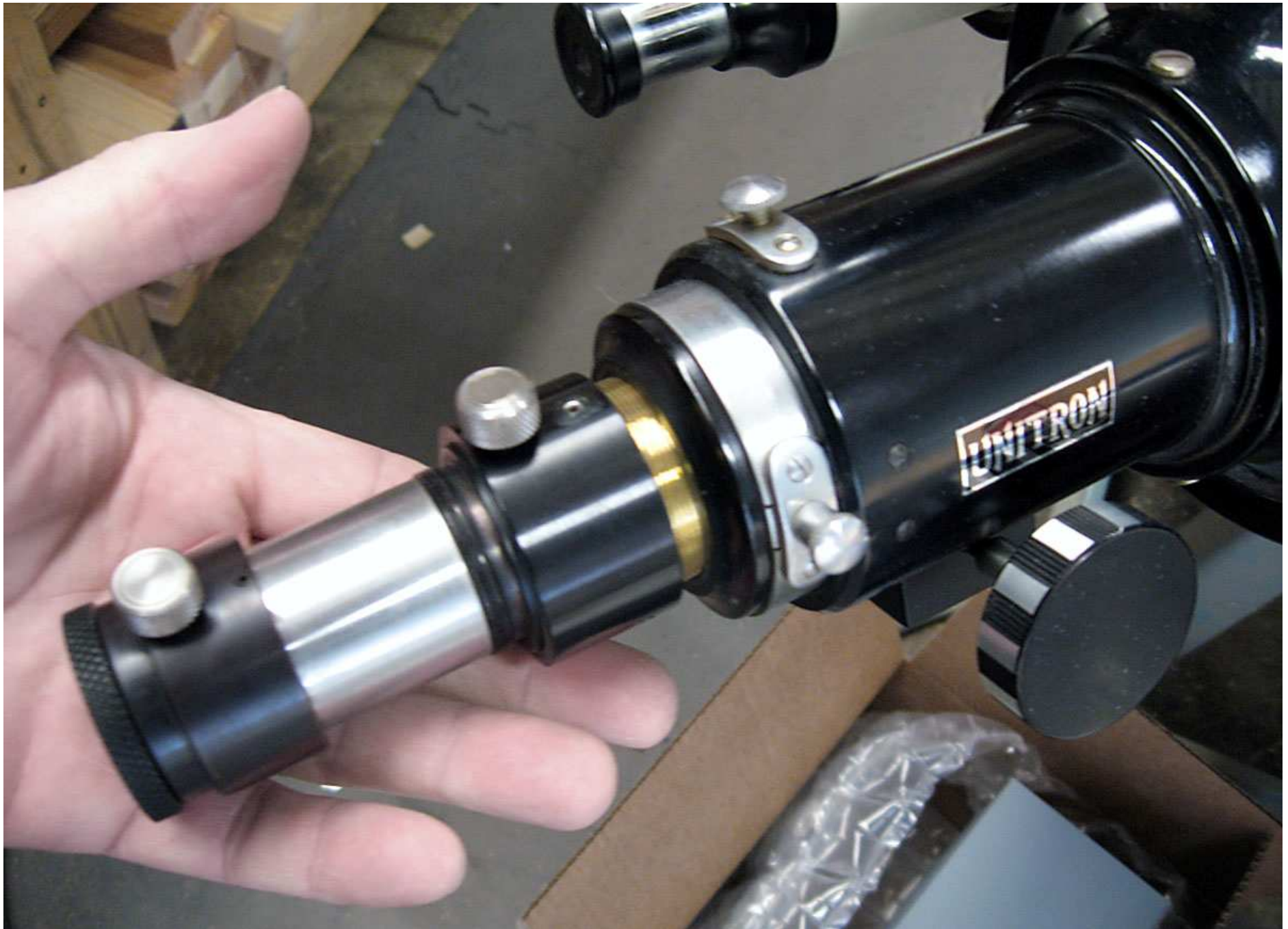
IMG_1670: Focuser on 6" OTA partially unscrewed to reveal Brass. From the weight, many fittings may be brass that is painted.
