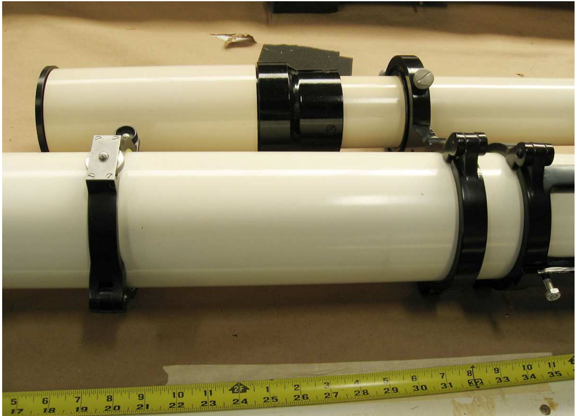
IMG_1687: 4" OTA & 3" guide scope. Note camera mount ring.
