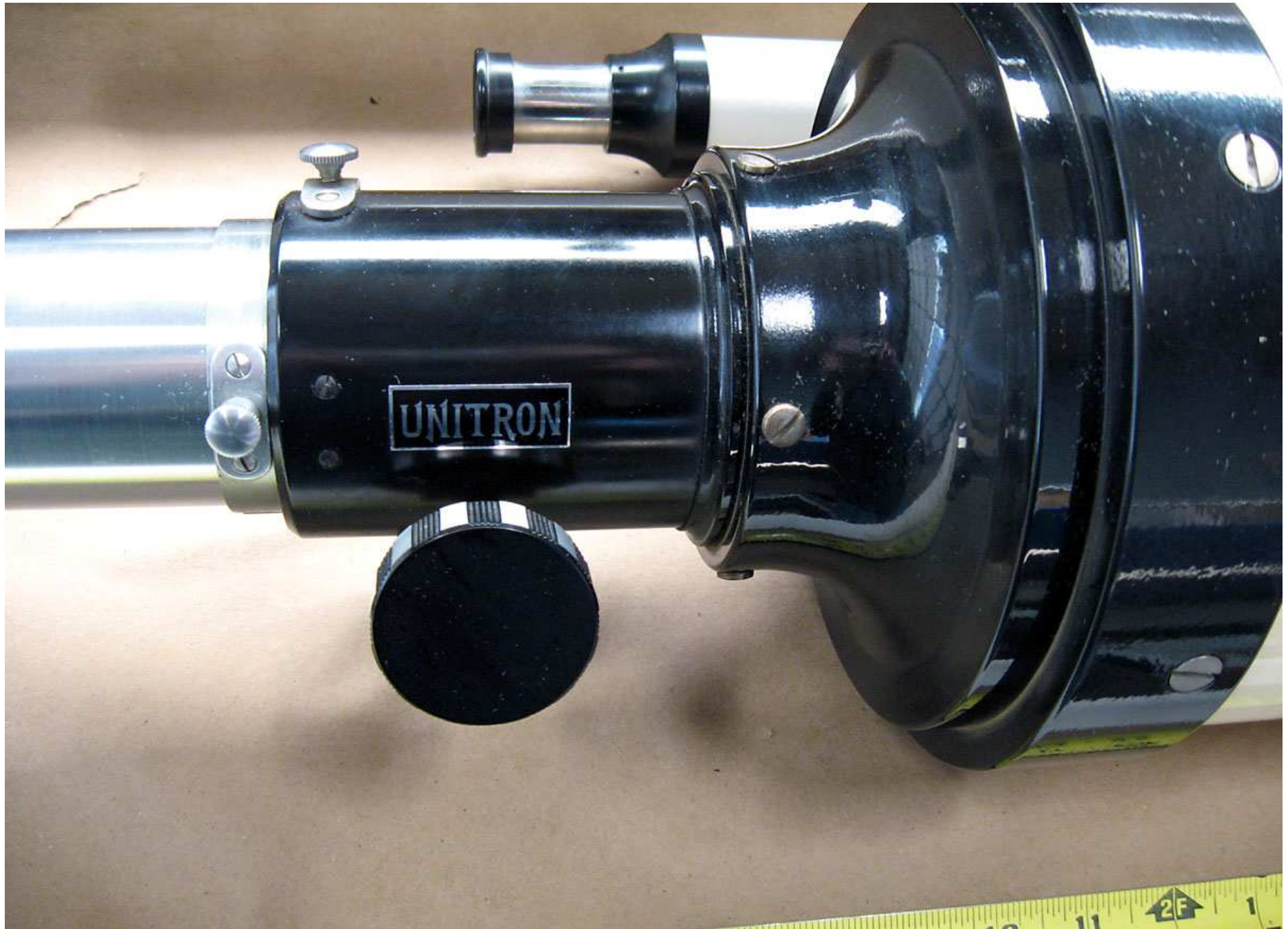
IMG_1648: Close-up view of 6" rear cell and focuser
