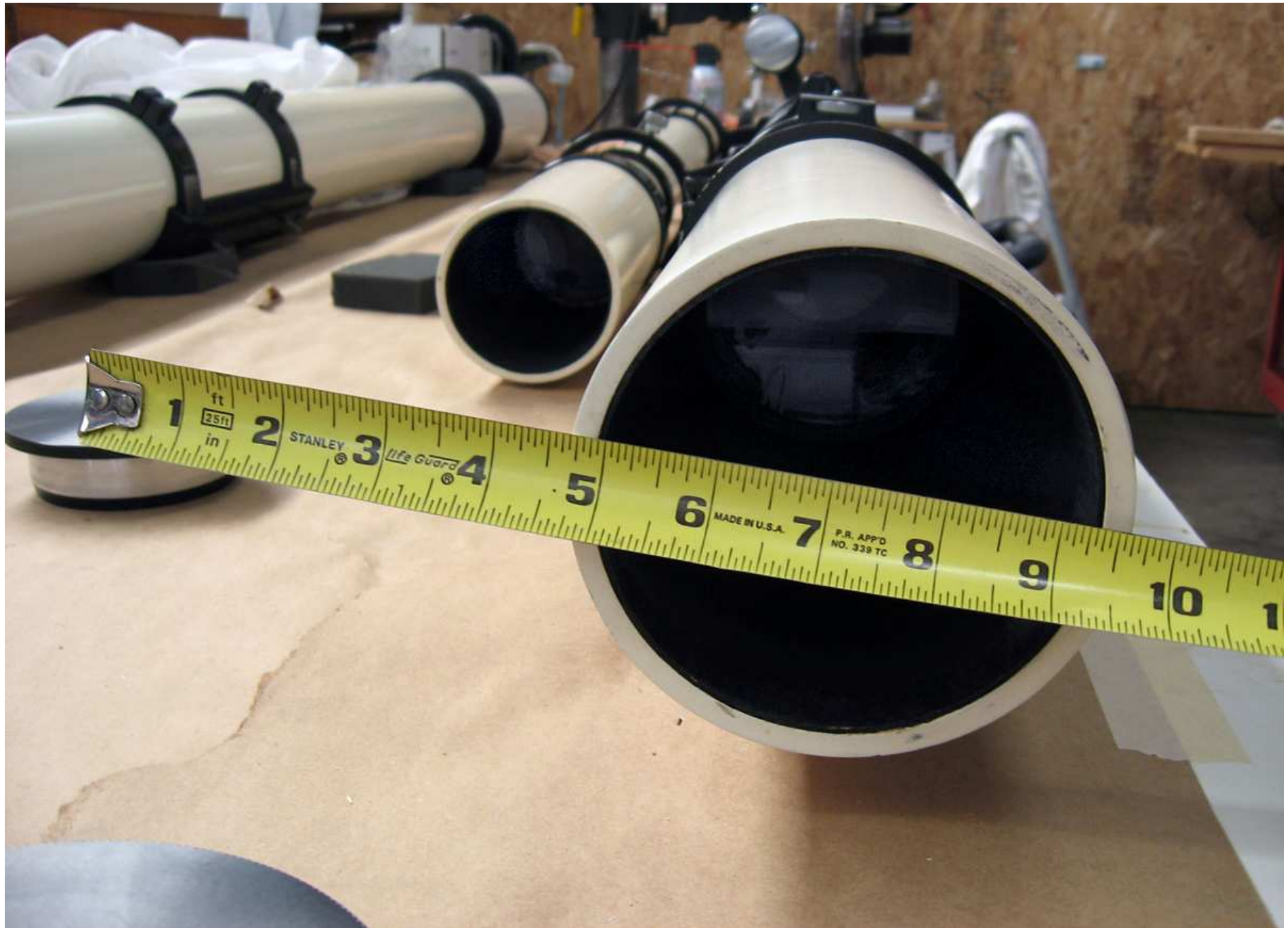
IMG_1697: 4" OTA with dew shield. Note how thick, some type of composite material.
