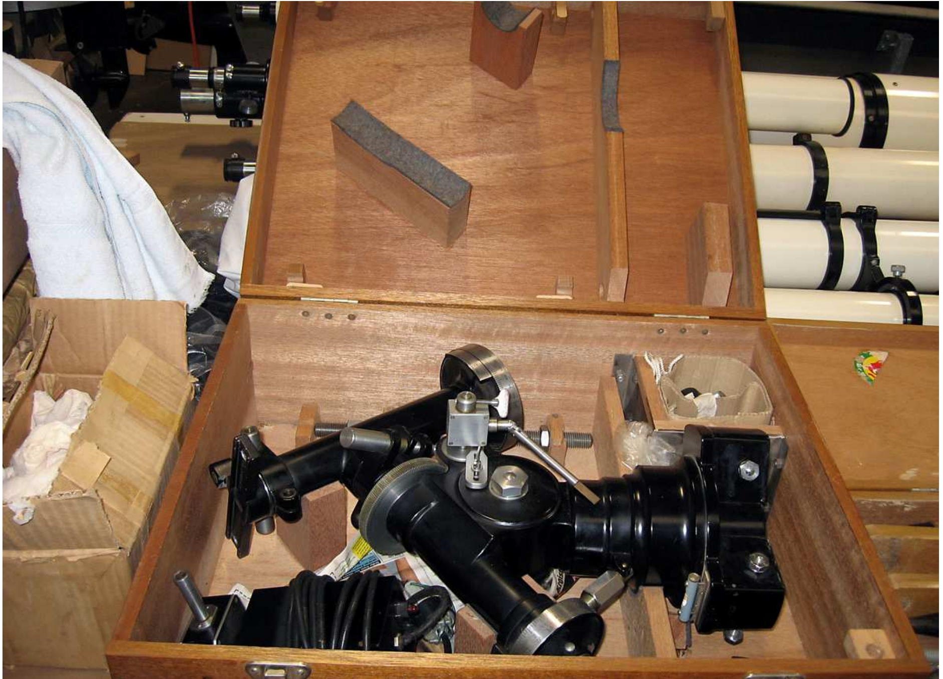
IMG_1630: What appears to be Unitron equatorial head, clock drive, OTA weights, etc., in Wooden Case.
