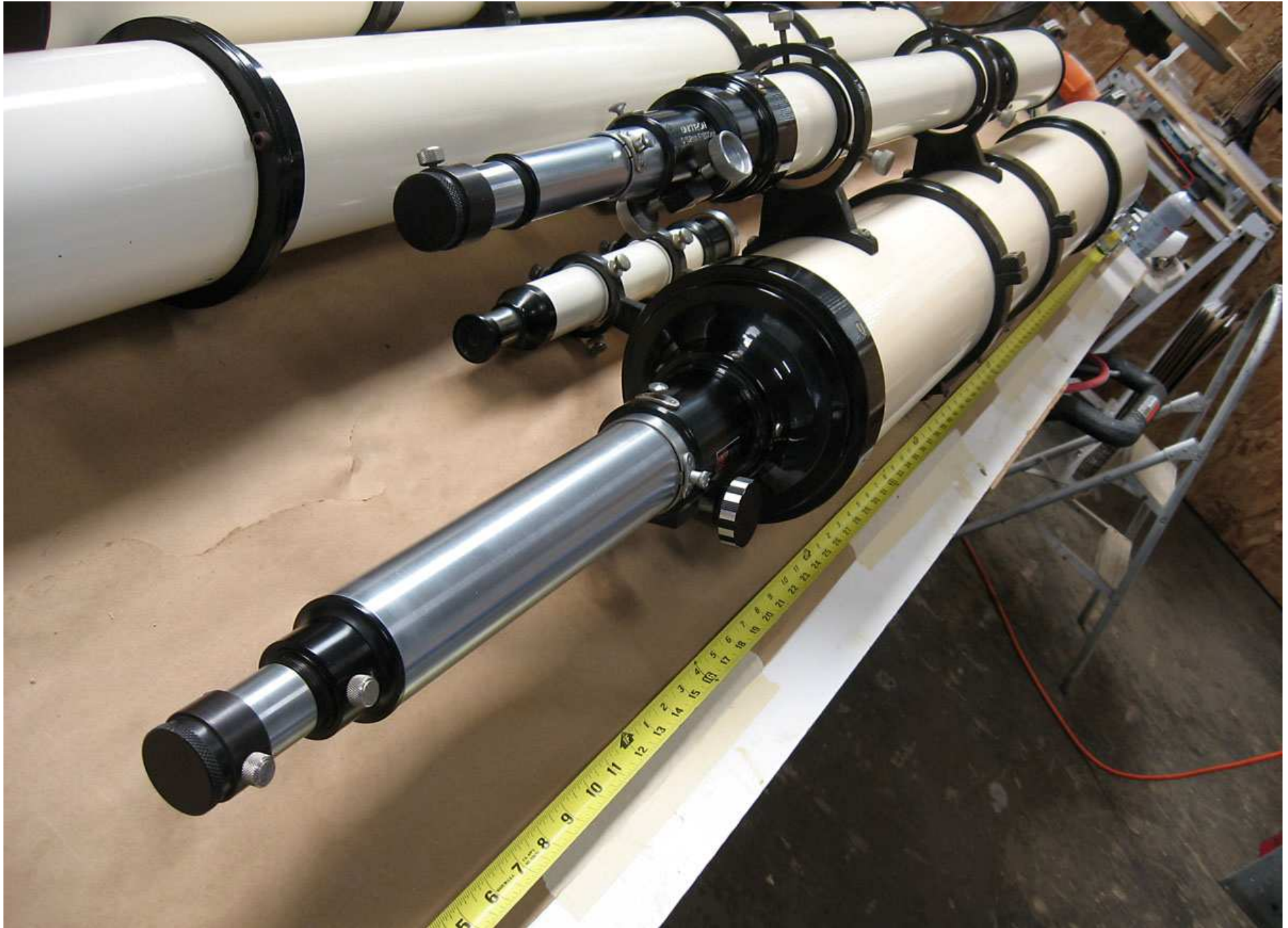
IMG_1647: 6" OTA with focuser extended on the main OTA & Guide-scope. Note finder and rings.
