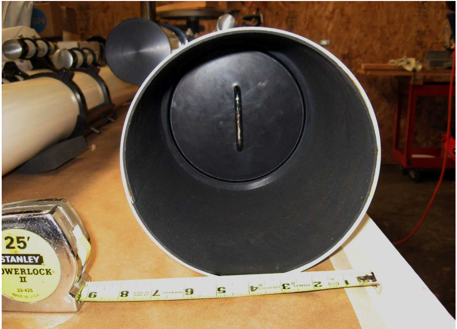
IMG_1641: Front of 6" OTA with metal objective cover. The handle shows some corrosion in the chrome finish.
