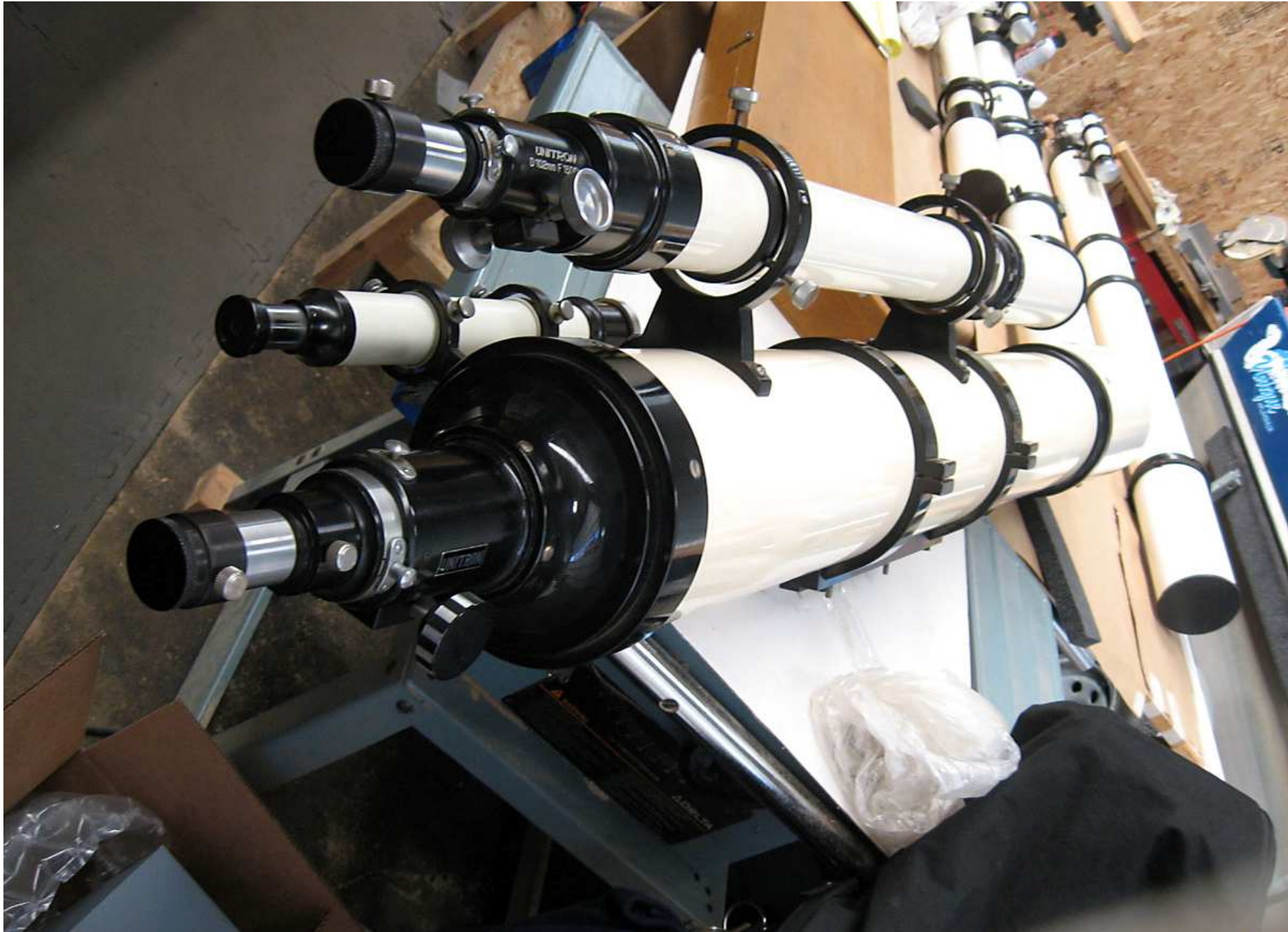
IMG_1667: Rear view of 6" OTA and attached scopes, pointed to the 5" OTA and the 4" OTA is on table with 3" guide scope & finder
