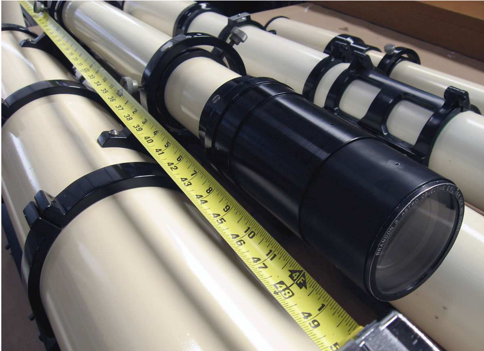
IMG_1655: Side view of Guide-Scope on 6" OTA, tape for scale.
