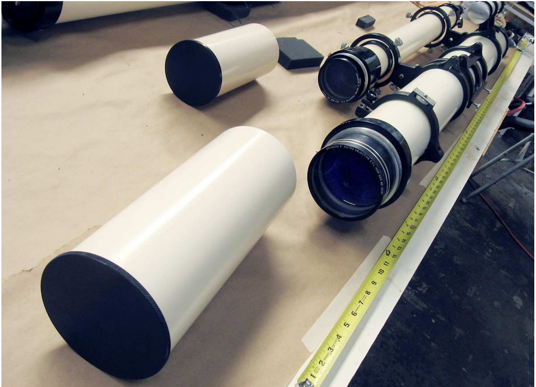
IMG_1693: 4" OTA showing slight blue on objective indicating some type of coating, as well as the 3" guide Scope.
