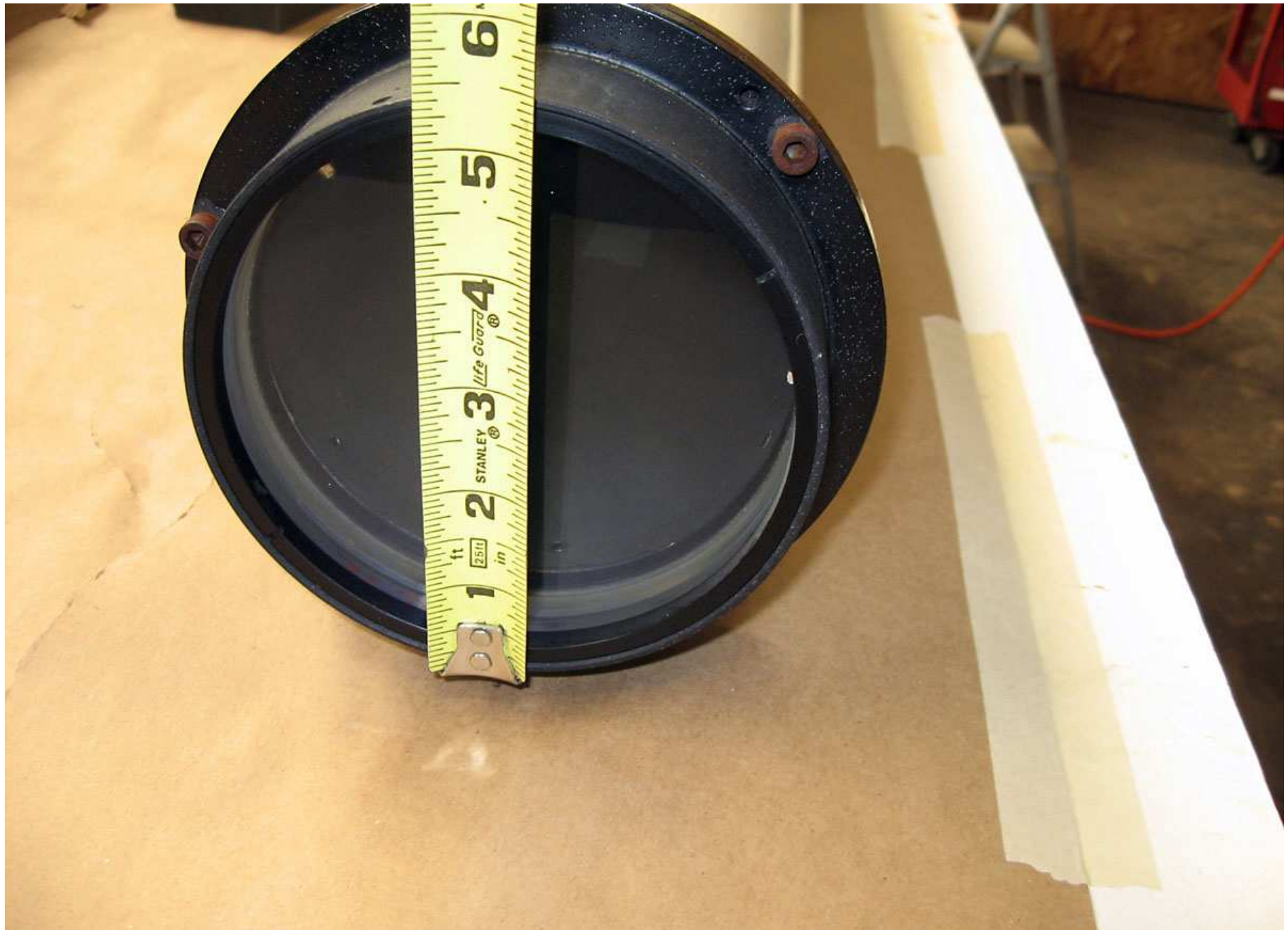
IMG_1677: 5" Objective with bright light to reveal very minor dust, better view of hex head screws & rust. No markings on Objective cell.
