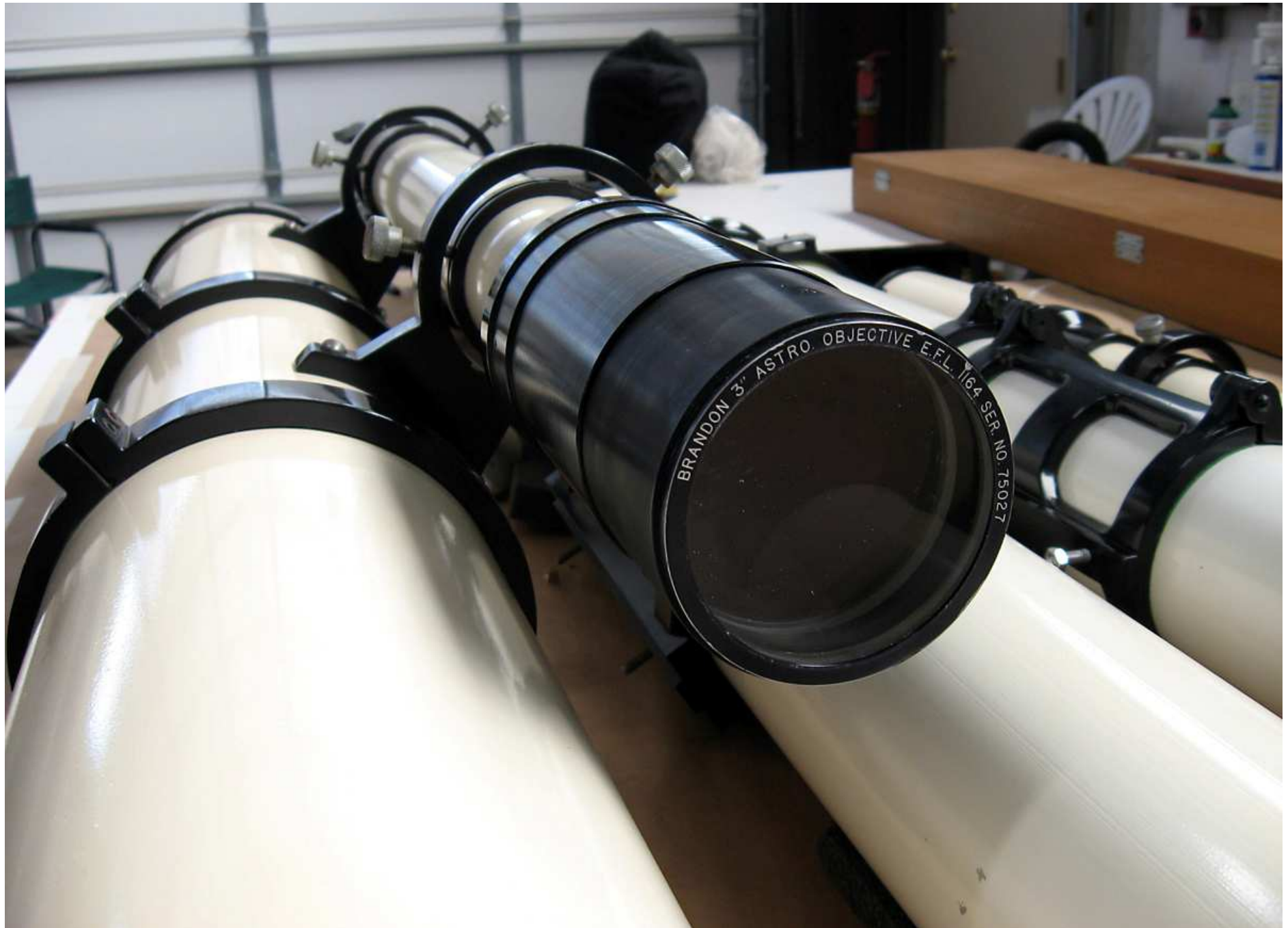
IMG_1652: same 3" guide scope with dew shield removed, some dust but no marks. 5" OTA on the right; note paint chips and paint lines
