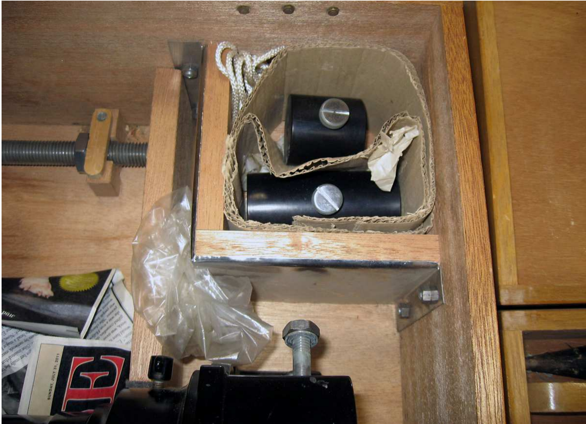
IMG_1631: Closer view of Equatorial box, OTA weights and threaded counter-weight shaft (no counter-weights)
