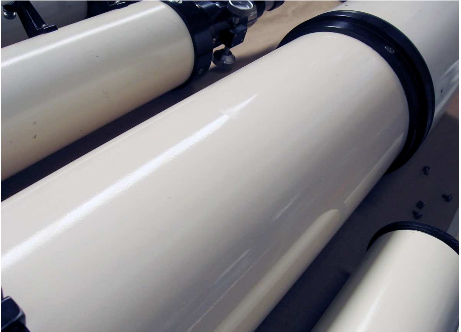
IMG_1660: 6" OTA. Note paint anomaly near top of reflection, there are a few spots like this on the OTA, "paint crinkle"
