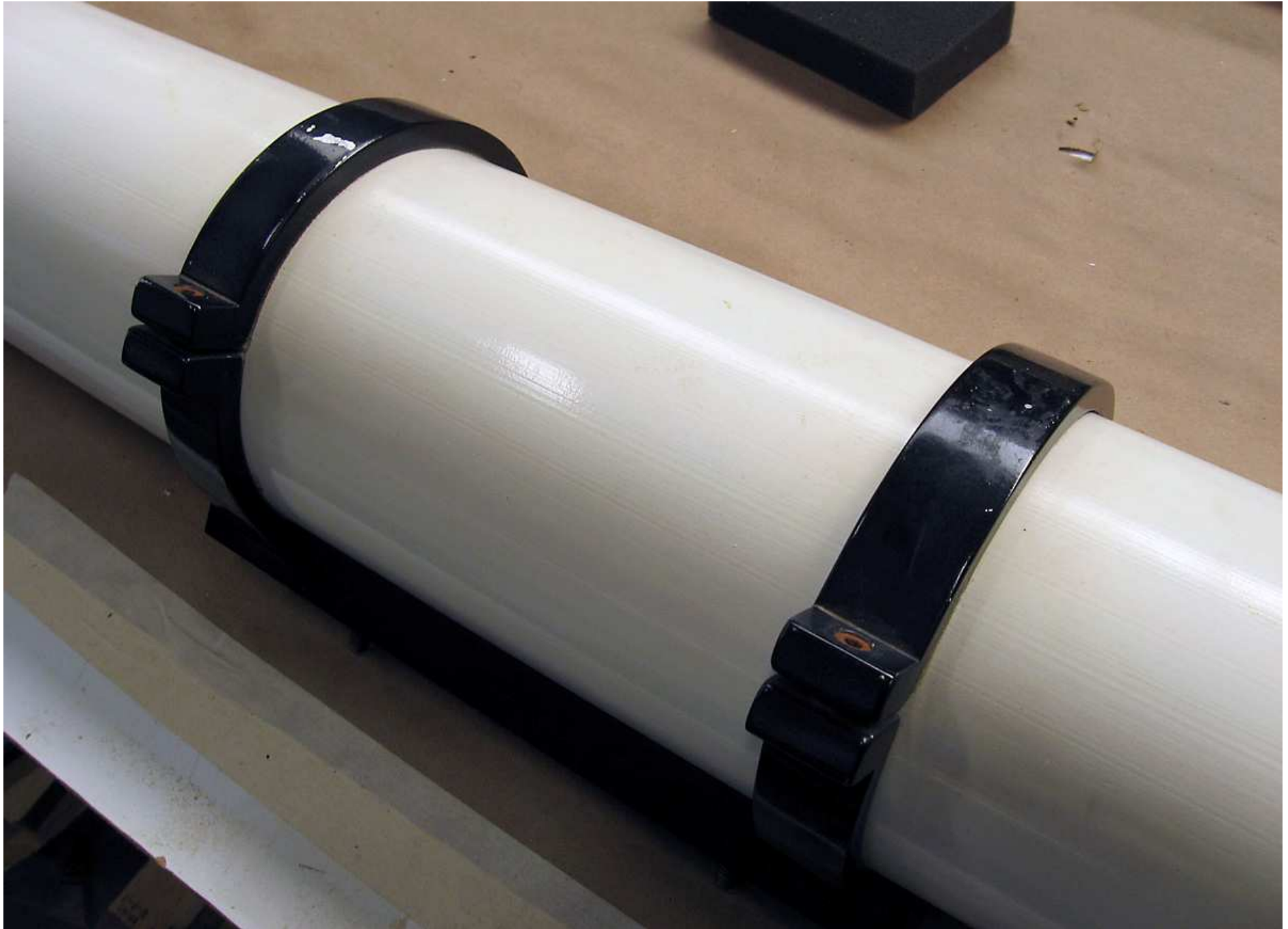
IMG_1679: 5" OTA rings, showing some paint flaking on them.
