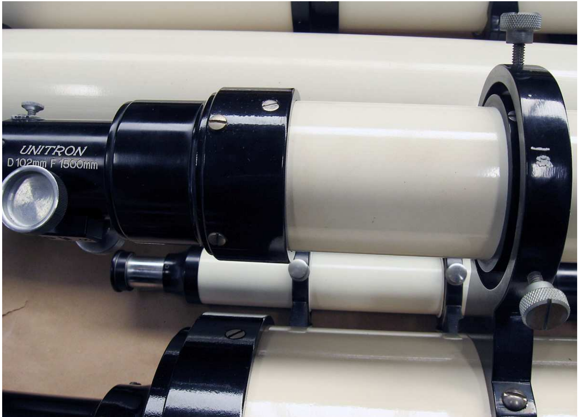
IMG_1658: Guide Scope on 6"OTA. Note rings and paint chips and oxidation on screws.
