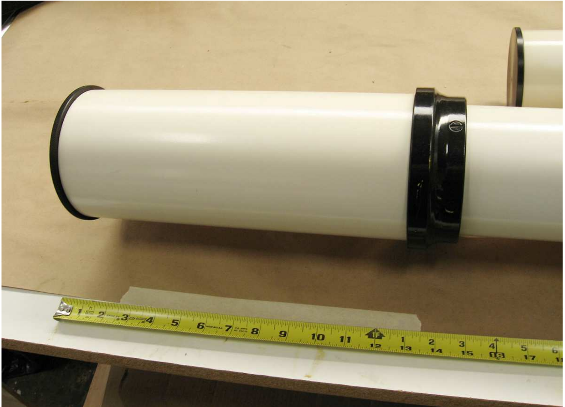
IMG_1686: Dew Shield and front of 4" OTA. This scope is very heavy in relation to the 6" OTA, being only 4"
