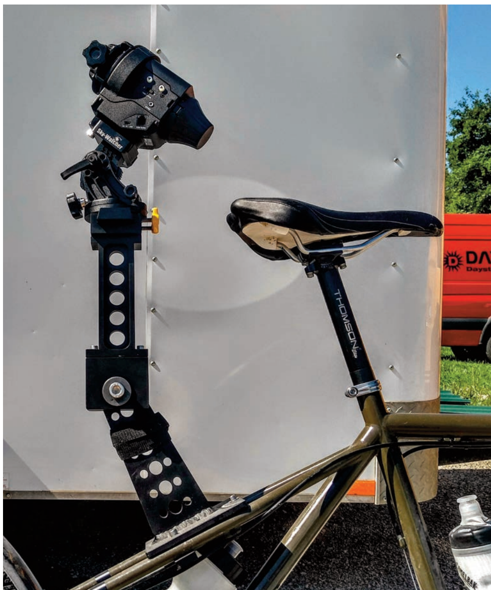
Image 2 - TSS's much improved remedy met the Big for the first time while at DayStar's Warrensburg, Missouri headquarters. The TSS system is comprised of five components: (1) a base, (2) a pivot block, (3) a riser, (4) a dovetail saddle and (5) a short Vixen-format dovetail rail.
