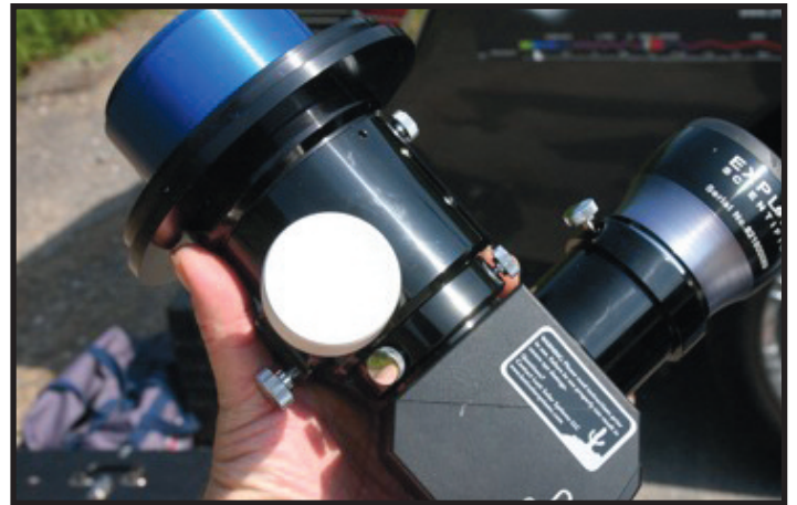
Image 4 – Set up as a white light/Solar Wedge scope.
