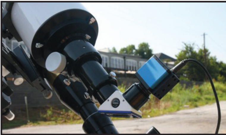
Image 3 - LS152mm scope in the with the CaK/white light module inserted.
