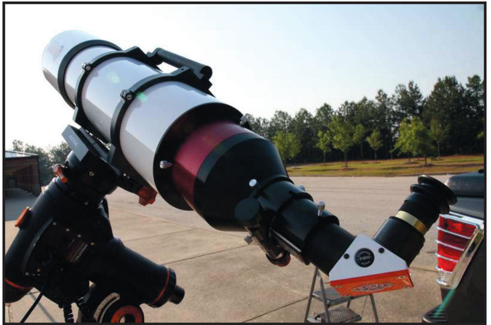
Image 2 - LS152 shown in H-alpha mode with B1800 blocking filter on CGEM mount.
