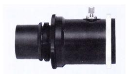
**16722 Standard Camera Adapter** — Provides a simple method by which a 35mm SLR camera body, less lens, is coupled to a telescope. It may be used for prime focus or eyepiece projection photography, and is adaptable to both 1¼-inch and 24.5mm i.d. eyepiece holders. Focusing is accomplished by means of the focusing mechanism of the telescope. Image size in projection photography is controlled by a set screw/lock nut mechanism.
