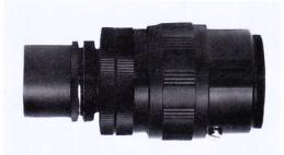
**16723 Deluxe Camera Adapter** — Provides a simple method by which a 35mm SLR camera body, less lens, is coupled to a telescope. It may be used for prime focus or eyepiece projection photography, and is adaptable to both 1¼-inch and 24.5mm i.d. eyepiece holders. Focusing is accomplished by means of the focusing mechanism of the telescope. Image size in projection photography is controlled by a helicoid mechanism.
