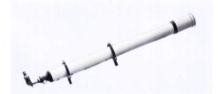
**60mm GUIDE SCOPE** — Complete with coated, airspaced, 2-element objective of 60mm clear aperture, 700mm focal length, focal ratio f/12, rack and pinion focusing mechanism, prismatic star diagonal, 9mm (78x) eyepiece with crossline, dewcap, dustcap and mounting brackets with centering screws for collimation.
