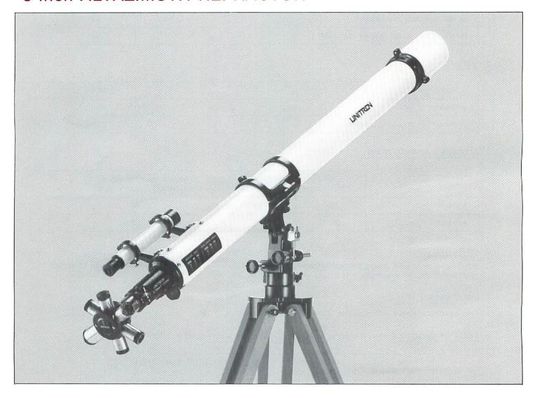
MODEL 140 — Complete with: altazimuth mounting with coarse and slow motion controls in altitude and azimuth; tripod with leg brace and accessories shelf; 8X-30mm viewfinder; Standard rack and pinion focusing mechanism with eyepiece holder; 5 coated eyepieces\*, 25mm (48X), 18mm (67X), 12.5mm (96X), 9mm (133X), 7mm (171X); dewcap; dustcap; wooden cabinet; instructions.
